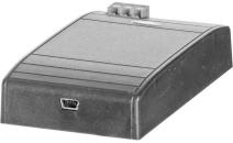
A 10 way DIP switch on the back of the unit is used to select the required output format. A green LED is used to indicate a successful data transfer and a red LED indicates an error condition.
