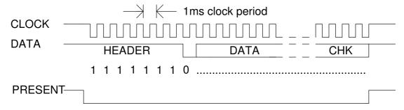
Data is set up on the falling edge of the clock and is stable on the rising edge of the clock.
