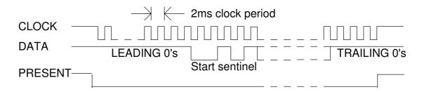
Each character is 5 bits long. The first four bits are the hex digit (0-F) least significant bit first. The fifth bit is an odd parity bit. A zero is represented by a high level on the DATA wire and a one is represented by a low level on the DATA wire. Data is set up on the falling edge of the clock and is stable on the rising edge of the clock. The PRESENT output goes low for the duration of the transmission simulating the CARD PRESENT from a mag card reader.
