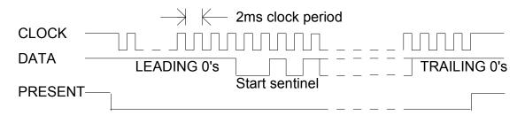
Each character is 5 bits long. The first four bits are the hex digit (0-F) least significant bit first. The fifth bit is an odd parity bit. A 0 is represented by a high level on the DATA connection and a 1 is represented by a low level on the DATA connection. Data is set up on the falling edge of the clock and is stable on the rising edge of the clock. The PRESENT output goes low for the duration of the transmission simulating the CARD PRESENT from a mag card reader.
