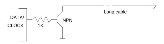
To ensure that the idle state of the transistor is off, the idle level from the module signal pins must be low. To achieve this connect INVERT to 0V.
