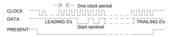
Each character is 5 bits long. The first four bits are the hex digit (0-F) least significant bit first. The fifth bit is an odd parity bit. A 0 is represented by a high level on the DATA wire and a 1 is represented by a low level on the DATA wire. Data is set up on the falling edge of the clock and is stable on the rising edge of the clock. The PRESENT output goes low for the duration of the transmission simulating the CARD PRESENT from a mag card reader.
