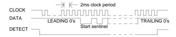
Each character is 5 bits long. The first four bits are the hex digit (0-F) least significant bit first. The fifth bit is an odd parity bit. A 0 is represented by a high level on the DATA pin and a 1 is represented by a low level on the DATA pin. Data is set up on the falling edge of the clock and is stable on the rising edge of the clock. The DETECT pin goes low for the duration of the transmission simulating the CARD DETECT from a mag card reader.
